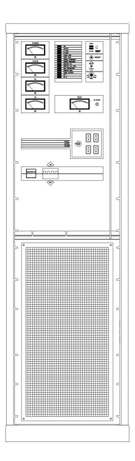
The T15000 is a power triode amplifier conceived for the FM band 88 - 108 MHz, with input and output frequency tuning.
