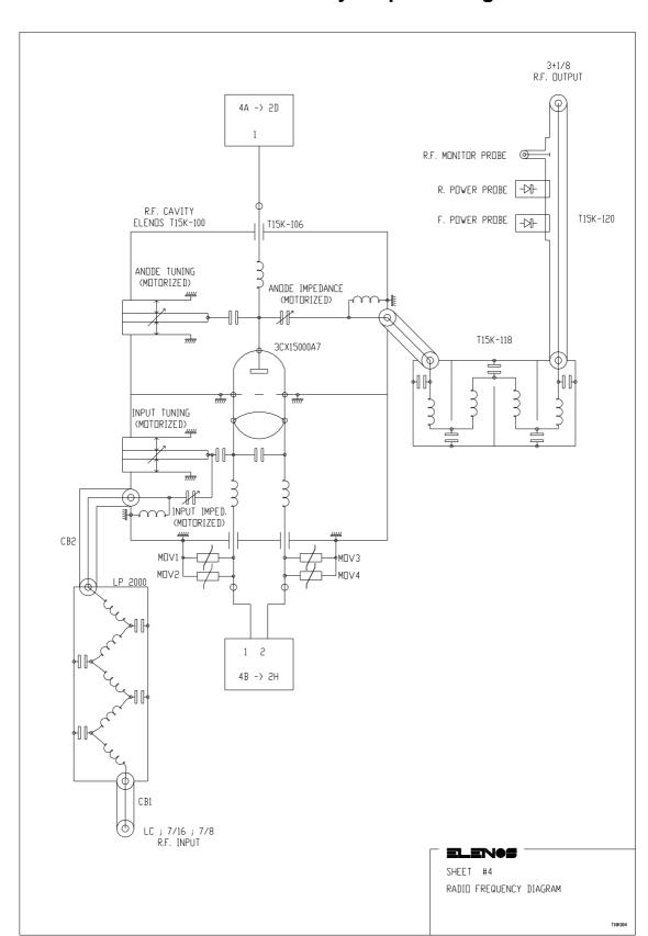
Sheet #4 - R.F. Cavity Amplifier Diagram
